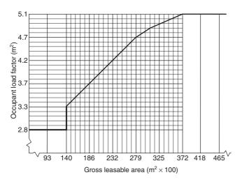
FIGURE 14.8.1.2(b) Mall Building Occupant Load Factors (SI Units). [101: Figure 7.3.1.2(b)]
