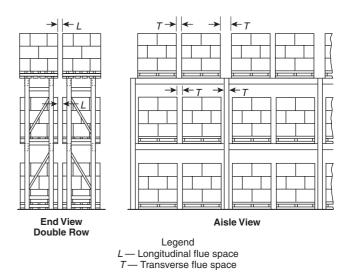
FIGURE A.34.7.3.1(a) Conventional Pallet Rack.
