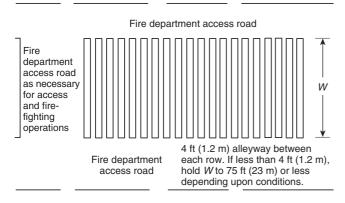
FIGURE A.31.3.5.3.1(b) Crib-Style Stacking into Solid Rows.
