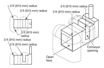
FIGURE 43.1.4.4.2 Class I, Division 2; Class I, Zone 2; Class II, Division 2; or Zone 22 Locations Adjacent to an Open-Face or Open-Front Spray Booth or Spray Room. [33:Figure 6.5.2]
