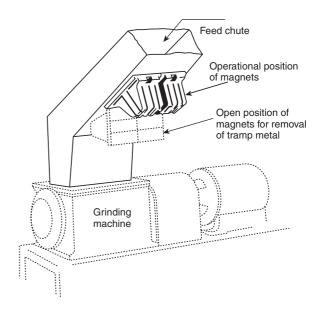
FIGURE A.40.4.1.2.3(b) Magnetic Separator. [654: Figure A.9.1.2.3(b)]
