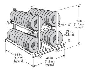
FIGURE A.34.8.1(c) Open Portable Tire Rack.
