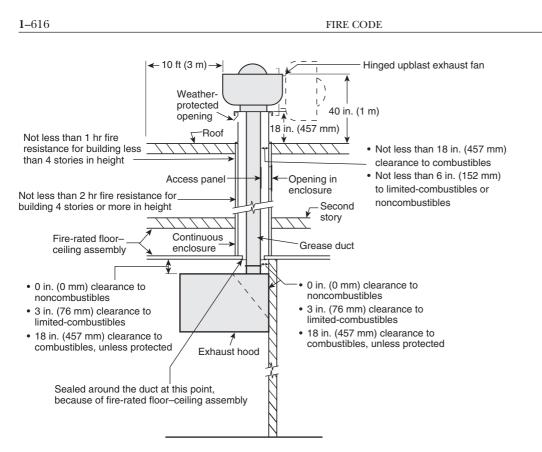
FIGURE A.50.2.2(a) Typical Section View for Building with Two Stories or More with Fire-Rated Floor–Ceiling Assembly. [96:Figure A.4.2(a)]
