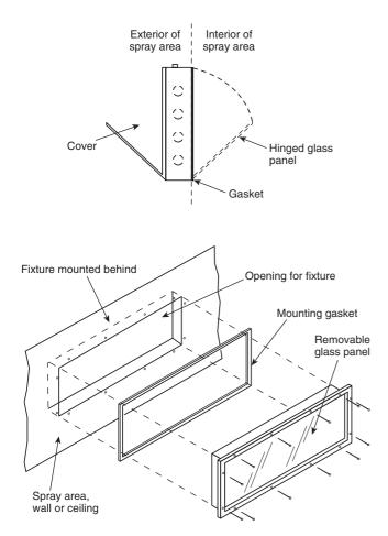
FIGURE 43.1.4.5.3 Examples of Light Fixtures That Are Integral Parts of the Spray Area and That Are Serviced from Inside the Spray Area. [33:Figure 6.6.3]
