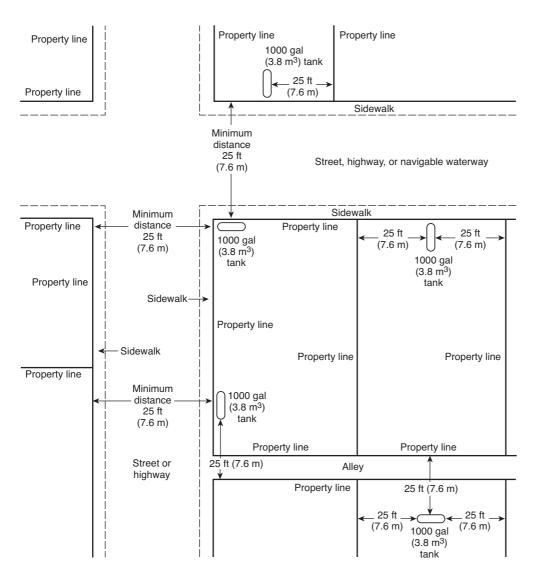
FIGURE A.69.3.3.1.1 Illustration of Separation Distances from Containers to the Line of Adjoining Property that can be Built Upon. [58:Figure A.6.3.1]
