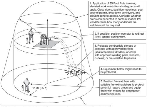
6. The PAI can extend the 35 Foot Rule as necessary (e.g., because of wind or elevation).
