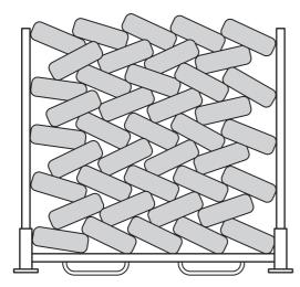
FIGURE A.34.8.1(g) Typical Laced Tire Storage.
