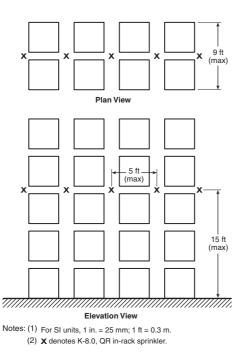
FIGURE 66.16.6.4(e) Double-Row Rack Sprinkler Layout H — Option #2. [30: Figure 16.6.4(e)]
