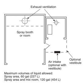
FIGURE 43.1.6.3.4(a) Mixing Room Within 6 ft (1830 mm) of Spray Area, Including Maximum Volume of Liquid Allowed. [33:Figure 8.3.4(a)]
