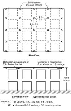
FIGURE 66.16.6.1.1(c) Multiple-Row Rack Sprinkler Layout for Design Scheme "A." [30: Figure 16.6.1.1(c)]
