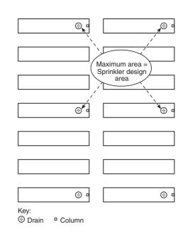
FIGURE A.66.16.8.2(d) Typical Arrangement of Floor Drains. [30: Figure A.16.8.2(d)]
