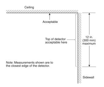
FIGURE A.13.7.4.3.3.1 Example of Proper Mounting of Smoke Detectors. [72: Figure A.17.7.3.2.1]
