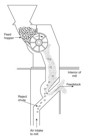
FIGURE A.40.4.1.2.3(a) Pneumatic Separator. [654: Figure A.9.1.2.3(a)]
