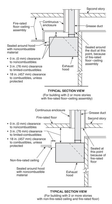
FIGURE A.50.2.2(e) Detail Drawings Showing Hoods Penetrating Ceilings. [96:Figure A.4.2(e)]
