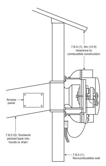
FIGURE A.50.2.2(f) Wall Mounted Fan. [96:Figure A.4.2(f)]
