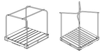
FIGURE A.34.8.1(b) Typical Palletized Portable Rack Units.
