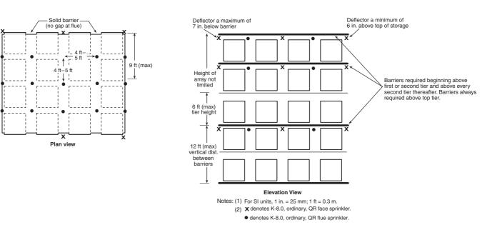
FIGURE 66.16.6.3.1(c) Multiple-Row Rack Sprinkler Layout for Design Scheme "C." [30: Figure 16.6.3.1(c)]
