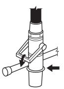
FIGURE A.13.6.4.6.2(e) Nozzle in Holder. [10:Figure A.7.6.2(e)]
