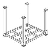
FIGURE A.34.8.1(a) Typical Open Portable Rack Unit.
