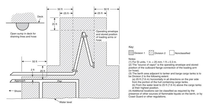
FIGURE 66.29.3.22 Area Classification for a Marine Terminal Handling Flammable Liquids. [30:Figure 29.3.22]
