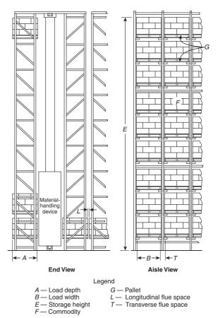
FIGURE A.34.7.3.1(e) Automatic Storage-Type Rack.
