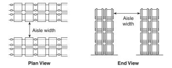
FIGURE A.3.3.7 Illustration of Aisle Width. [13:Figure A.3.9.3.1]
