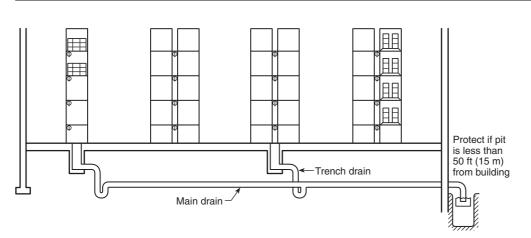
FIGURE A.66.16.8.2(a) General Scheme for Warehouse Spill Control of Liquids. [30: Figure A.16.8.2(a)]
