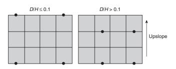
FIGURE A.13.7.4.3.3.4.5 Spot-Type Detector Spacing for Sloping Ceilings with Beam Pockets. [72: Figure A.17.7.3.2.4.5]
