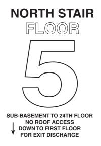
FIGURE A.10.11.3 Example of a Stairway Marking Sign. [101: Figure A.7.2.2.5.4]
