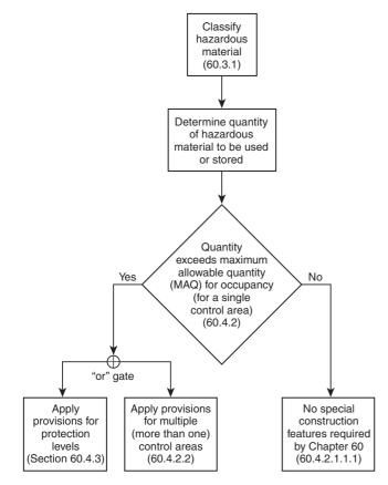
FIGURE A.60.4.1 Application of Chapter 60 Requirements for Hazardous Materials. [400:Figure A.5.1]
