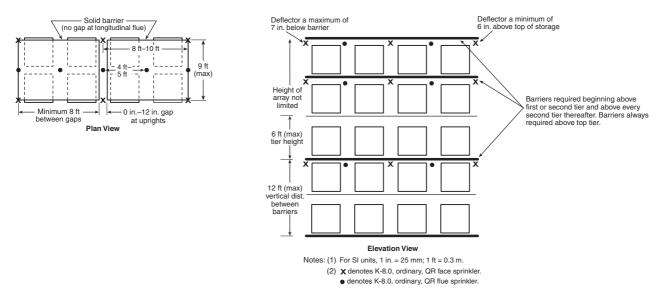
FIGURE 66.16.6.3.1(b) Double-Row Rack Sprinkler Layout for Design Scheme "C." [30: Figure 16.6.3.1(b)]
