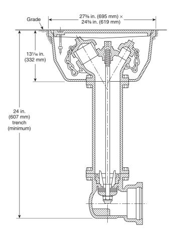
FIGURE A.3.3.121(b) Flush-Type Hydrant. [25:Figure A.3.3.12(b)]
