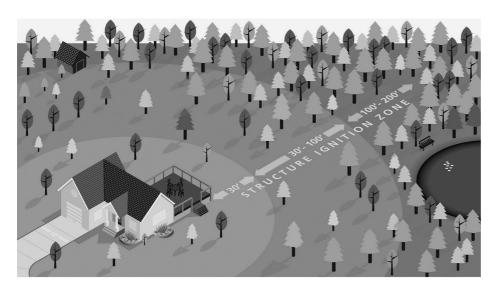
FIGURE A.17.1.8 The Structure Ignition Zone. [1144:Figure A.4.2.4]
