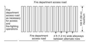
FIGURE A.31.3.5.3.1(a) Relatively Open Stacking Methods.
