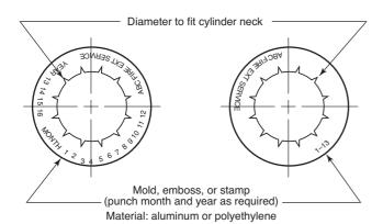
FIGURE A.13.6.4.10 Design of a Verification-of-Service Collar. [10:A.7.10]
