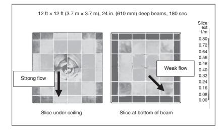
FIGURE A.13.7.4.3.3.4.2(3)(a) Reservoir and Channeling Effect of Deep Beams. [72: Figure A.17.7.3.2.4.2(3)(a)]
